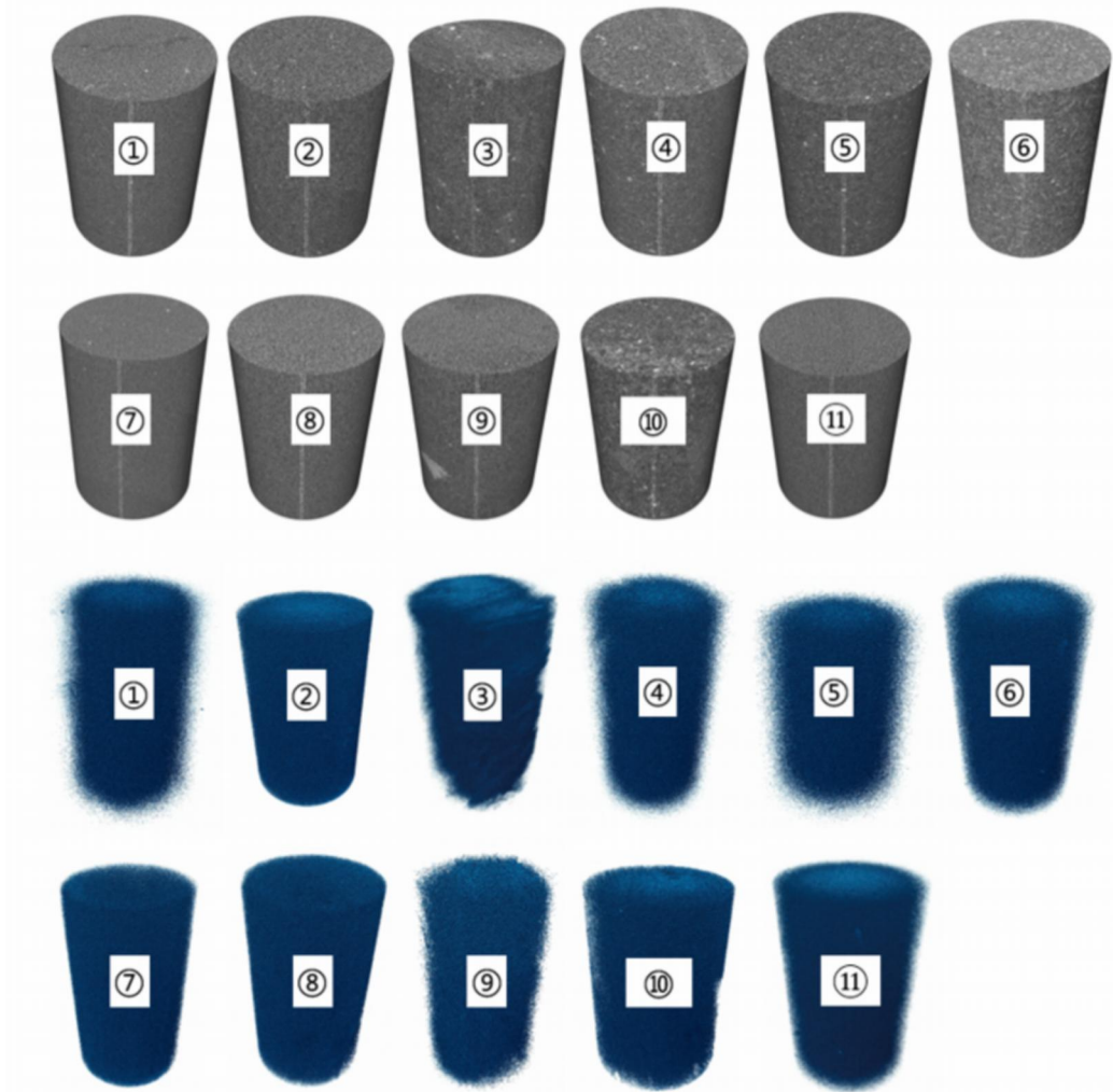
Fig. 6 Three-dimensional CT data and pore structure of tight sandstone core samples
