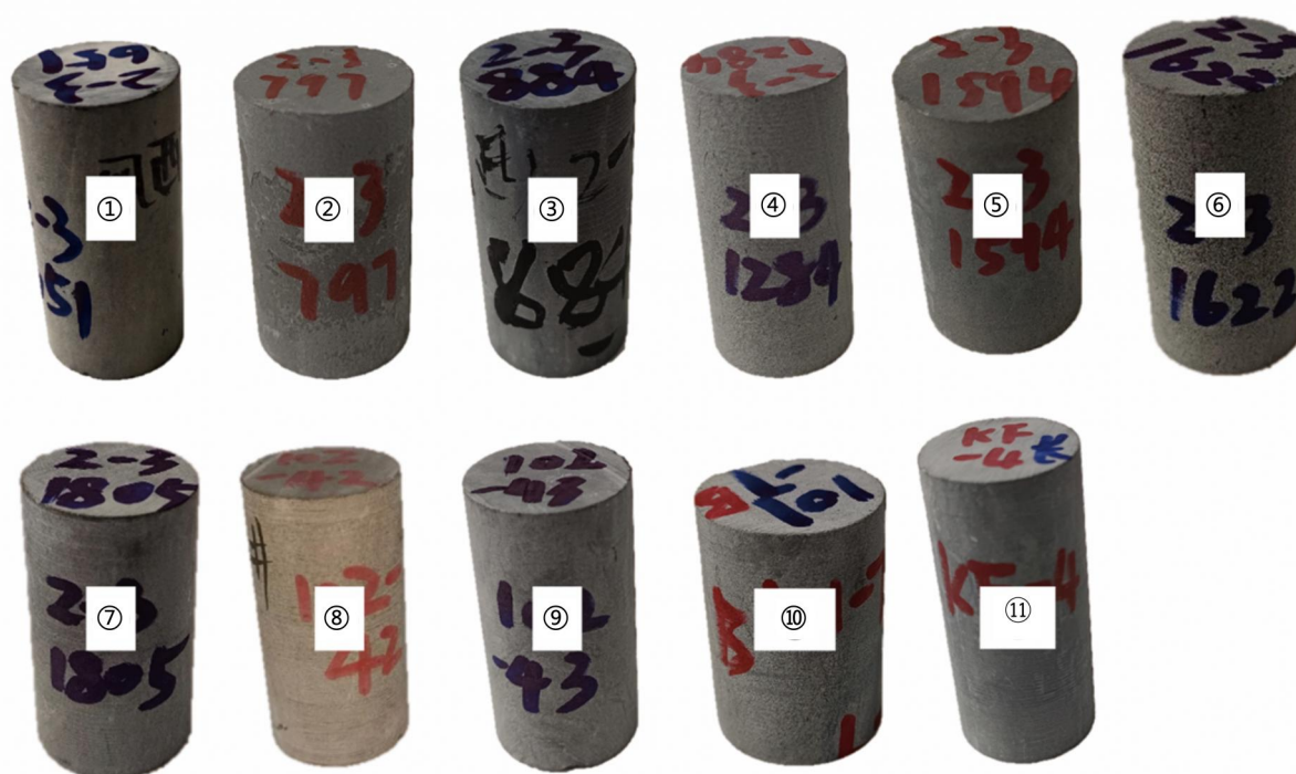
Fig. 5 Tight sandstone core sample
