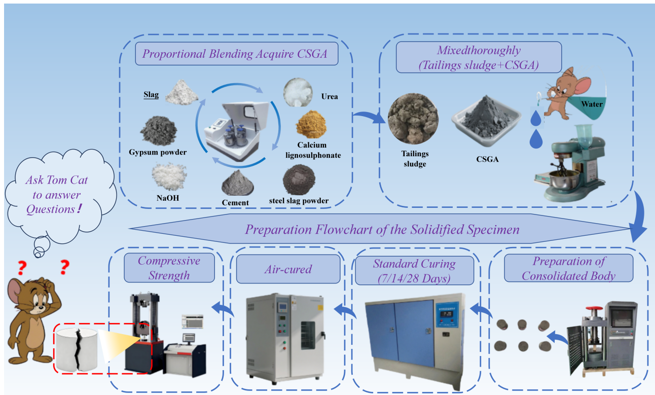
Fig. 1 Flow chart of the solidified body preparation process
