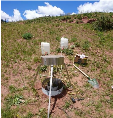
Fig. 5 The slope infiltrometer at the test field
