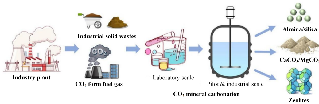
Fig. 8 Schematic diagram of CO 2 mineralization by industrial wastes (Chen et al., 2021)
